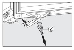
Caution. Do not move the front part of the soft-close mechanism in the direction shown when the restraining clip ② has been removed.
